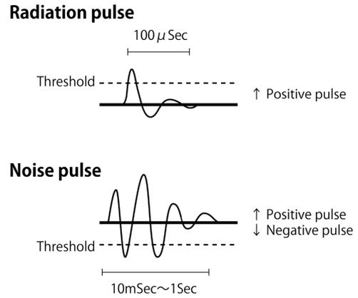
Fig. 4. Detection mechanism for noise and radiation pulses.
