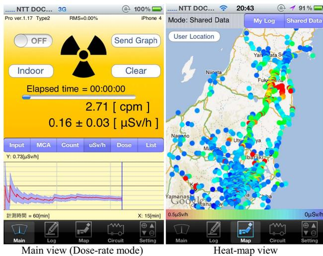
Fig. 5. Screen captures of the POKEGA application: main view (dose-rate mode), heat-map view, oscilloscope mode, MCA mode, counting log mode, and total dose mode.
