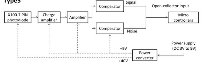
Fig. 2. Block diagrams for Types 1 through 5.
