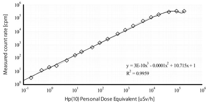
Fig. 6. POKEGA measurement range using  $^{137}\text{Cs}$ .
