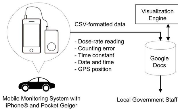
Fig. 8. Mobile radiation monitoring system with Pocket Geiger.
