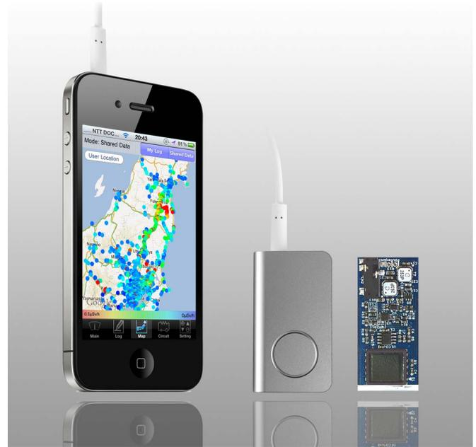
Fig. 1. Pocket Geiger (Type 4) and its PCB.
